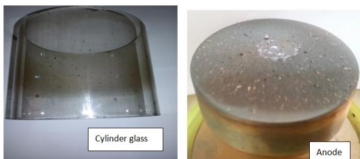
Figure 5 shows pictures from the cathode and the anode and the cylinder glass after each arc discharge
