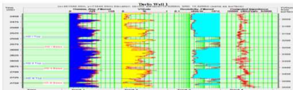
Fig. 4.0: Derby well showing suite of logs used in identifying prospective reservoirs
