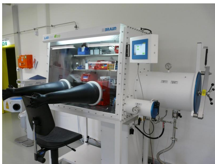
Fig. 3 Preparation of the nano-composites was done under protective atmosphere in a glove box.
