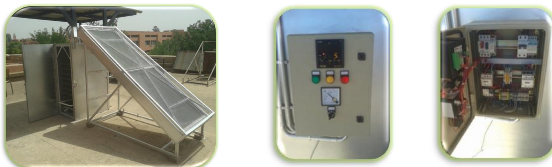
Figure 1. Partially solar dryer running in forced convection (EESPAM) with the control box.
