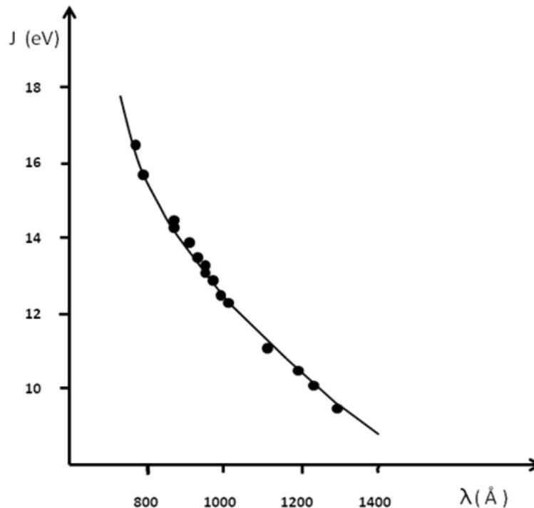
**Fig 7:** The influence of the ionization energy  $J$  versus the threshold wavelengths of the photoelectric effect. 19 different gases have been studied. (Reproduction from Ref 17)
