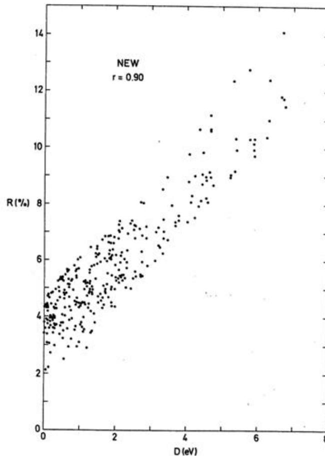
**Fig 1** Plot of fluctuation data R versus  $D(E) = J^a - J^b + h\nu_{mn}^a - h\nu_{kl}^b$ . (difference of ionization energy plus photon energy) from fifteen steel samples used in a hollow cathode lamp. Seventeen elements were studied in this graph. (Reproduction from Ref 4)
