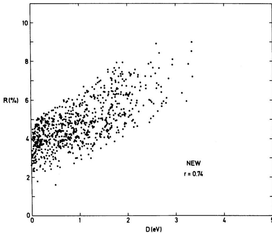
**Fig 2:** In the analyses of Fig 2 39 spectral iron lines in the wavelength region 240 - 750 nm were simultaneously and repeated measured 30 times with the ICP - IDES system. Reproduction from Ref ( 1 ).
