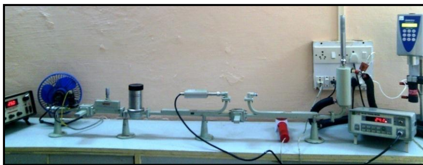
Figure 1. The experimental setup of microwave X-band bench for the measurement of \epsilon' and \epsilon''
