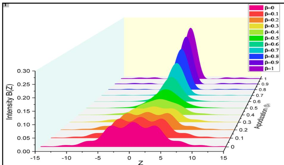
**Figure3. 3D Waterfall Graph: Intensity Distribution of Four-Zone Amplitude PSF with defocus  $\phi_d=2\pi$  and primary spherical aberration  $\phi_s=2\pi$**
