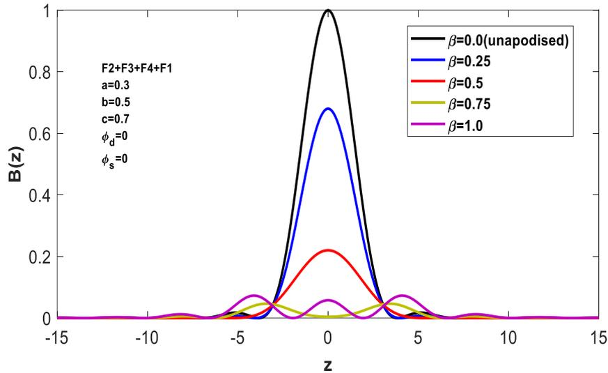
**Figure 1. Point Spread Function (PSF) Intensities without Defocus and Spherical Aberration**
