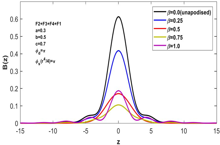
Figure 2. PSF Intensities with Defocus  $\phi_d=\pi$  and Spherical Aberration  $\phi_s=\pi$  for varying apodization parameters ( $\beta$ )
