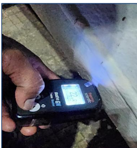
Fig.4: Confirmation of radiotracer passage at SV-3
