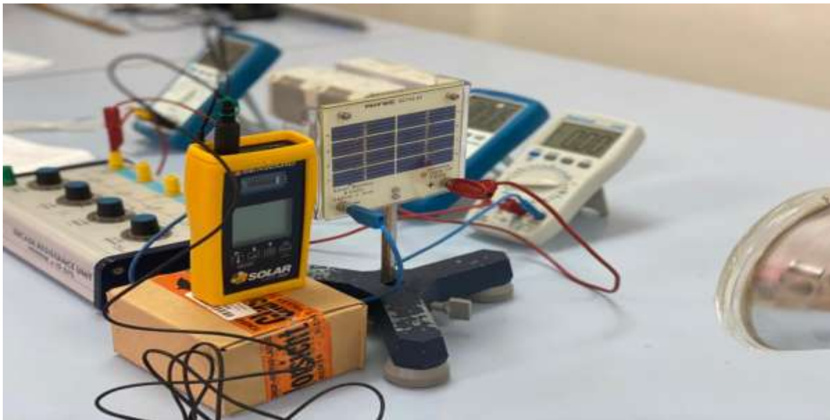
Fig. 1: Experimental labels: (i) Mono crystalline cell (ii) Polycrystalline cell, and (iii) Circuit system.
