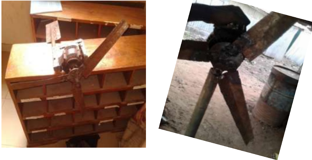
Figure 5: Coupled Alternator, Turbine, Frame and Galvanized Pole
