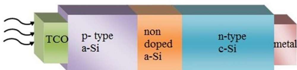
Fig. 2 Hetero junction with intrinsic thin layer Solar cell
