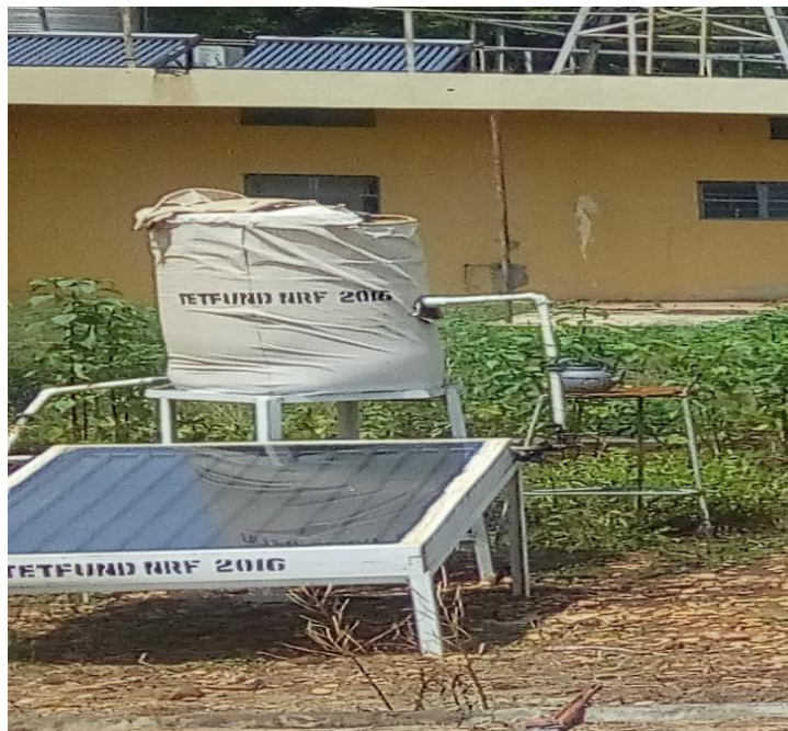
Plate 2: Flat plate collector solar water heater
