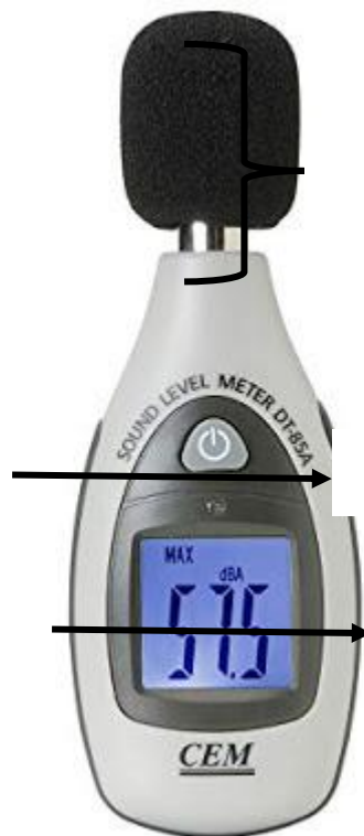
Figure 1. Simple Digital Sound Level Meter
