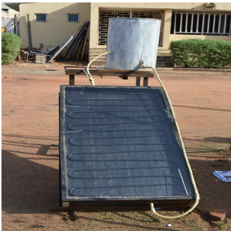
Figure 2. Closed view of thermosyphon solar water heating system.
