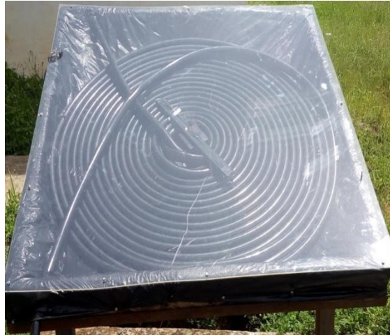
Figure 3(a): Black hose solar collector
