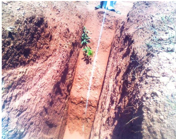
Figure 4 Trench in the study area for profile sampling of different litho units.
