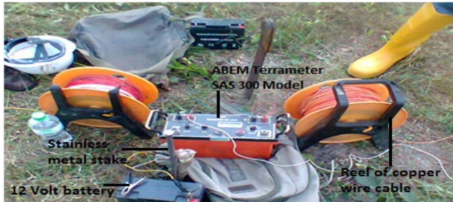
Fig. 2: Set of Vertical Goelectric Sounding (VES) Equipment for Data Acquisition
