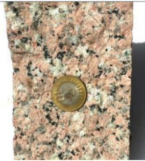
Photograph 8: Showing the Coarse grained, equigranular variety of granite (Sample JB6).
