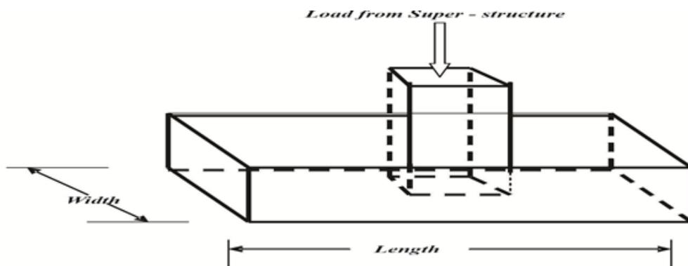
**Fig. 7:** Schematic of dimensions of an Isolated Footing
