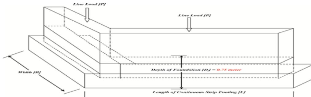
**Fig. 8:** Schematic of dimensions of a Continuous Strip Footing
