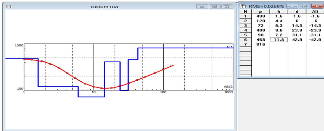
Fig. 3: Geo-electric model generated for VES data
