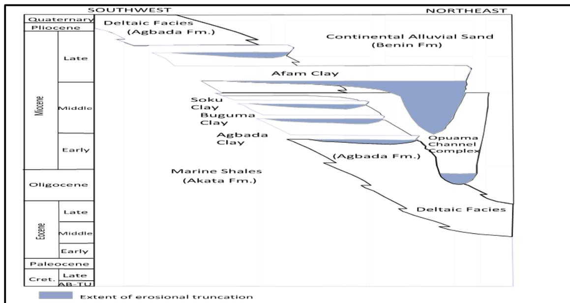
Figure 1: Stratigraphic column showing the three formations of the Niger Delta<sup>2</sup>
