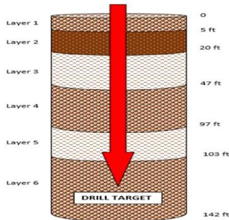
Fig. 4: Schematic of Geo-electric layers showing target aquifer
