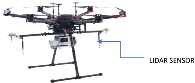
Figure 1 - RPA MATRICE 600 with LiDAR Source: GVI (2023).
