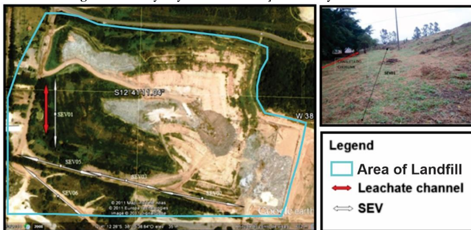
Figure 6: Survey Layout in the Camaçari Sanitary Landfill Area.
