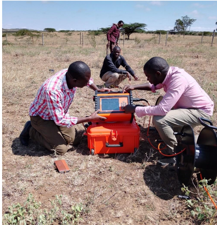
Figure 2.1: Resistivity Data Acquisition process using LS 2 ABEM terrameter
