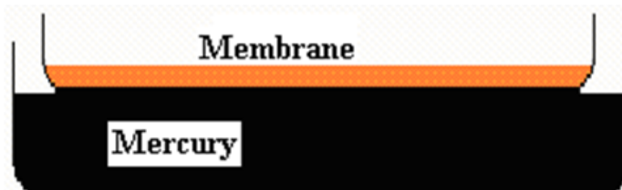
Figure 1:-Schematic figure of the petri dish floating on a mercury tray
