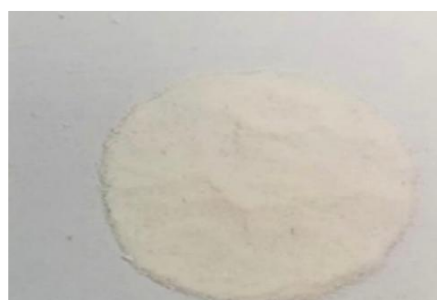
Fig. 2. Rice husk-derived silicates synthesized through controlled calcination and alkali extraction method, showing the formation of amorphous nano-silica with high purity due to the naturally high silica content of rice husk biomass.
