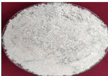
Fig. 1. Maize husk-derived silicates prepared under similar green synthesis conditions, illustrating comparatively lower silica yield and the presence of minor impurities influenced by the initial biomass composition.
