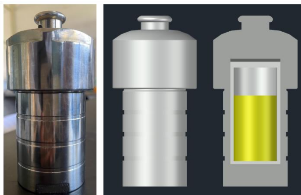
Figure 1 Autoclave reactor for solvothermal synthesis
