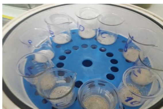
Figure 2: Recipients with dry residues for the cooling period. Source: Author.
