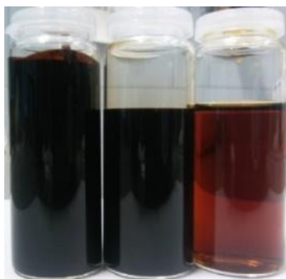
Fig. 4. (L-R): original black liquor, retentate and permeate at pH 10
