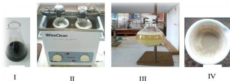
Figure 1: Synthesis of ZnO NPs using TDLE; I- TDLE, II- incubation in a sonicator, III- after 2 h and IV- synthesized ZnO NPs.
