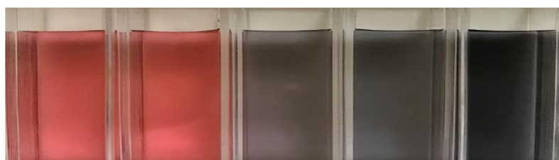
Figure 2: Photograph of color change of pet food samples spiked with different concentrations of melamine. (From left to right: 0 ppm, 0.10 ppm, 0.25 ppm, 0.75 ppm, and 1.50 ppm).
