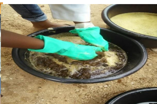
Plate 2.2: Washing of Pulped Sample to Remove the Black Liquor
