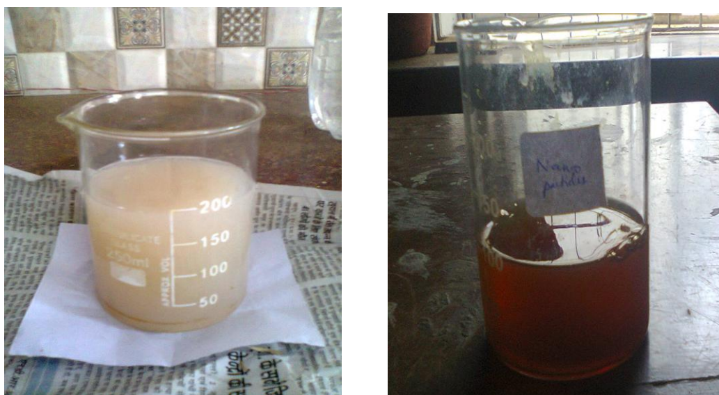
Fig. 1 The conversion of silver nitrate to nano silver by A.marmelos after 24hrs.
